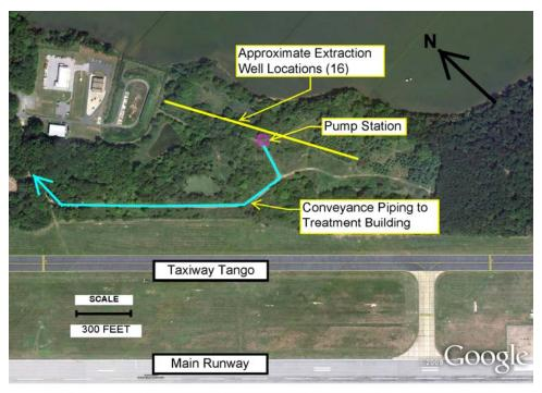
FIGURE 1 - CURRENT 30% DESIGN PUMP STATION AND PIPING LAYOUT (TREATMENT BUILDING AT AN OFF-AIRPORT LOCATION)
